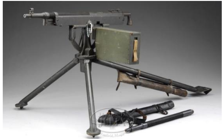
Colt-Browning M1895/14 Machine Gun, made by Marlin Corp. Image courtesy of James D. Julia Auction House.
